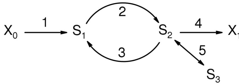
$$\begin{aligned}\frac{dS_1}{dt} &= v_1 - v_2 + v_3 \\ \frac{dS_2}{dt} &= v_2 - v_3 - v_4 - v_5 \\ \frac{dS_3}{dt} &= v_5\end{aligned}$$
