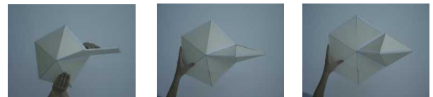
Figure 2: Deformation of the Goldberg icosahedron (Fig 1, right). Left: in one extreme position: the right unit is completely flat. Centre: in the neutral position, both units have the same shape. Right: in the second extreme position, the left unit is completely flat.
